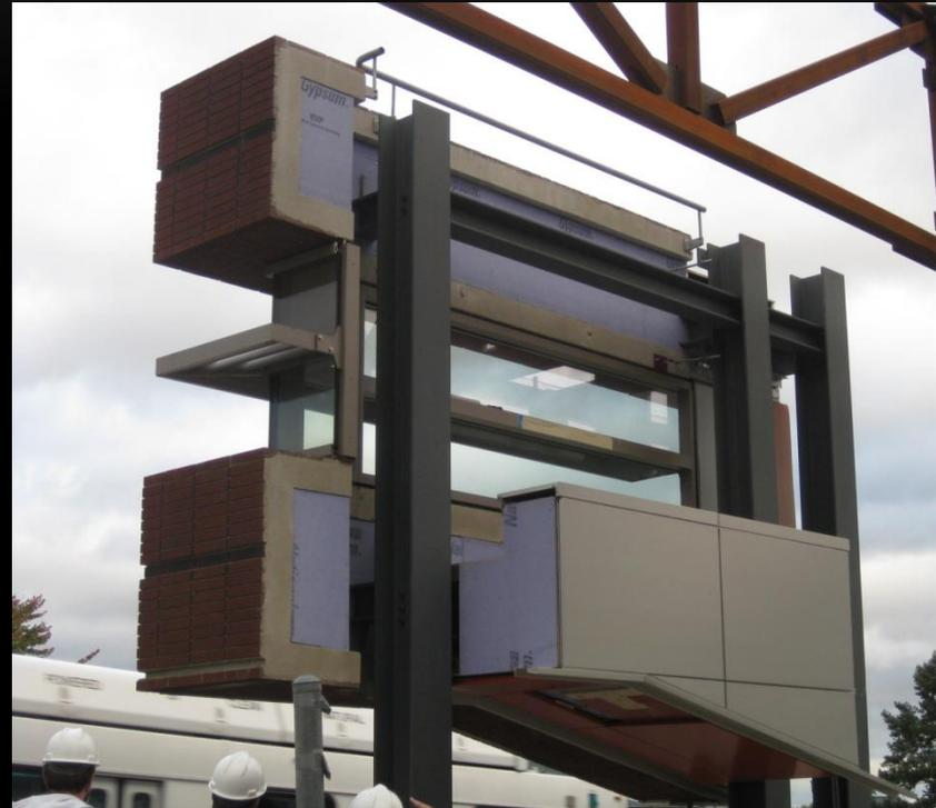
Phase change material applied within drywall and the glazing affects temperature swings and impacts daylighting in spaces.
